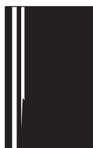
White lines in sub scan direction
